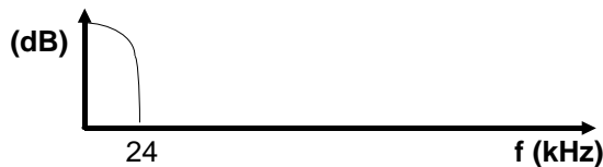
Figure 26. Spectrum After Continuous Time Filter
